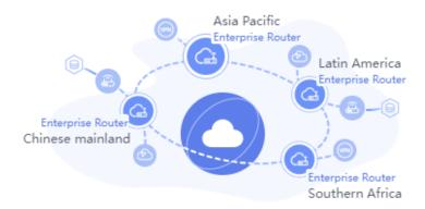
Communication between on-premises data centers and the cloud across regions: Enterprise routers and global DC gateways are added to a central network as attachments, so that on-premises data centers can access the cloud over the Huawei Cloud backbone network.
